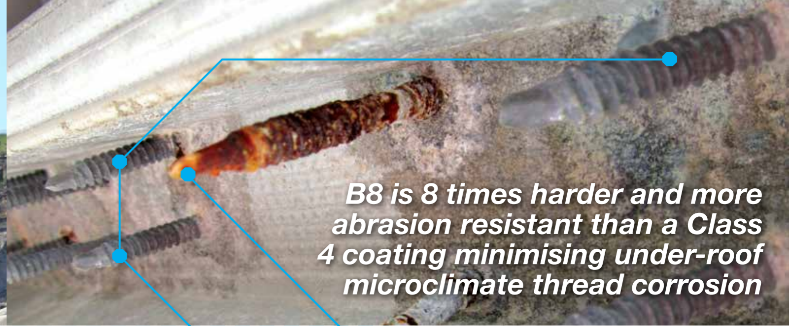
Conventional Class 4 Mechanically Galvanised Screws
